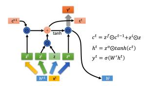
Figure 1: The internal structure of LSTM
